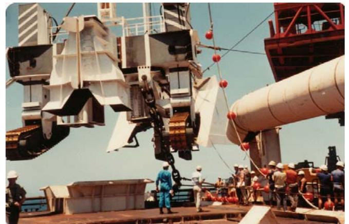
1983 - Woodside's North Rankin A-to-Dampier pipeline 450 te. plough being deployed for the first time.
