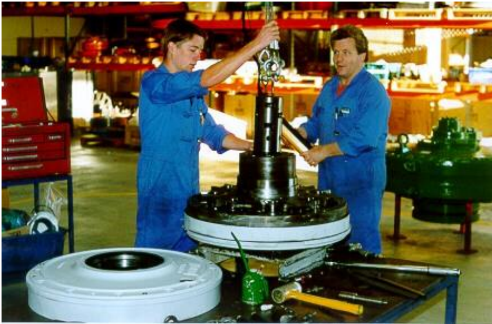
Hagglunds Drives apprentice Leon Griffiths (left) and technician Tony Adams repairing a Hagglunds Viking motor. This photo was taken in Hagglunds Drives WA workshop circa 1990, although the exact date is unknown.
