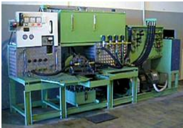
Prior to dispatch each pump and motor is tested on Hydraulic Resource's test bench to ensure performance integrity.
