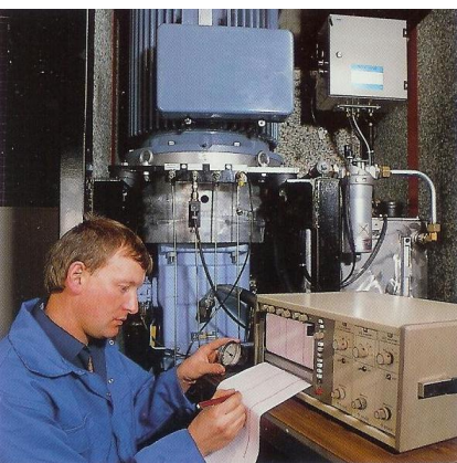
A young Chris on site data logging a Hagglunds Drives power unit
