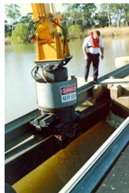
A recent application used a DIN module to control the vertical movement of a lock crane boom. Located on the River Murray in South Australia is a series of locks for flood control. Concrete beams are lowered into slots to vary the height of underwater barriers.
